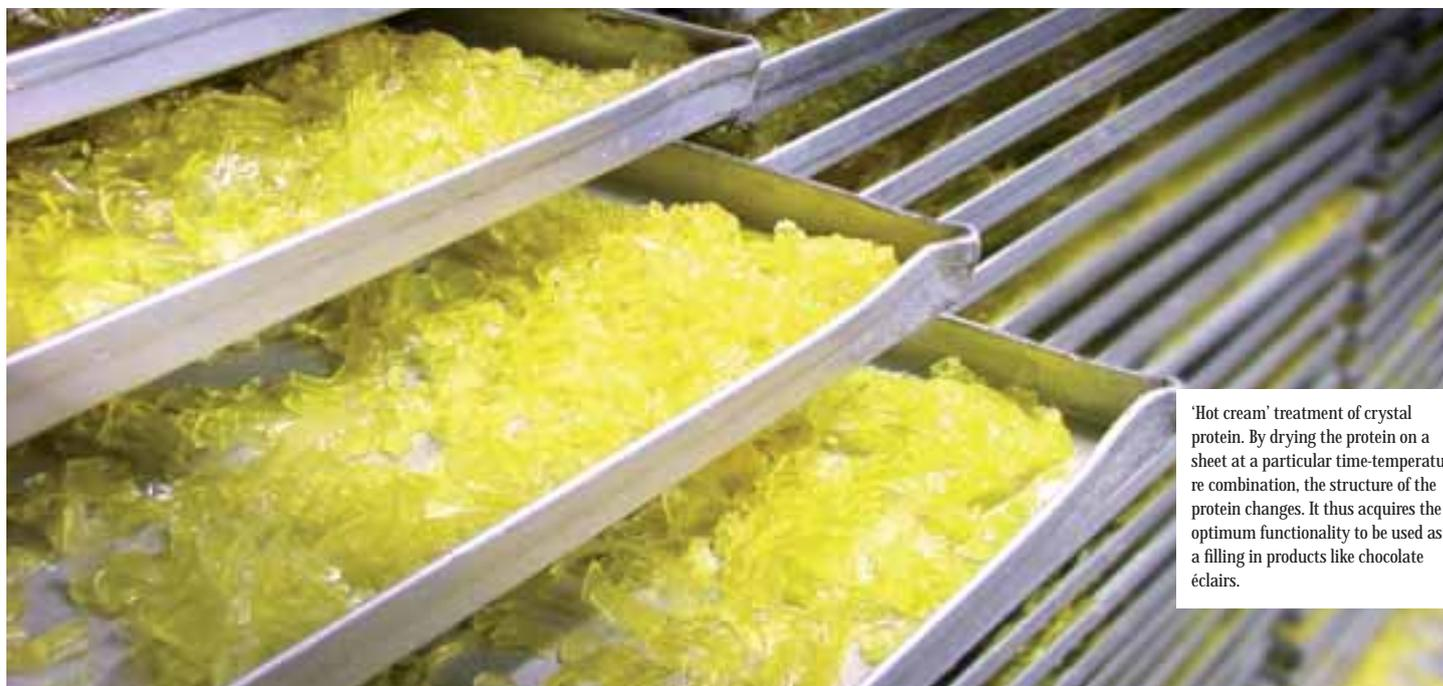
'Hot cream' treatment of crystal protein. By drying the protein on a sheet at a particular time-temperature combination, the structure of the protein changes. It thus acquires the optimum functionality to be used as a filling in products like chocolate éclairs.
